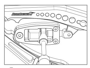
(3) Align everything properly before compressing the punch to remove the pivot ball.
