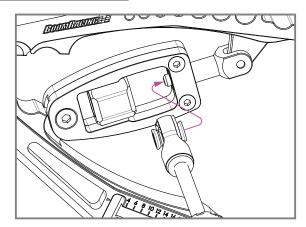
Position the rod end or shock absorber so that the side you want to punch the pivot ball out from is facing the die side.
