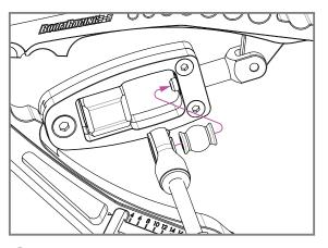
2 Insert the pivot ball on the side from which you want to punch it in. Ensure the pivot ball is facing the punch side.
