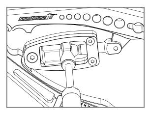
3 Align all components carefully before compressing the punch to install the pivot ball.
